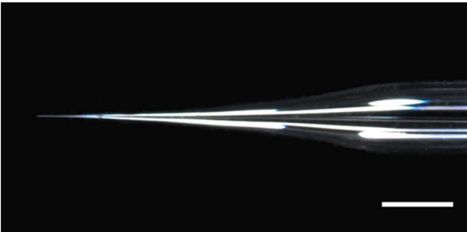
**Figure 4. Glass needle used for puncturing blastomeres during the ablation procedure.** The needle shown here was pulled on a Sutter P97 needle puller using a program with parameters 2 x (heat = 566, pull = 100, velocity = 20, time = 250) + 1 x (heat = 566, pull = 100, velocity = 100, time = 250). Other instruments or programs may be used to pull needles suitable for ablation, as long as they are of the same general shape as the one shown here. Scale bar = 1 cm.
